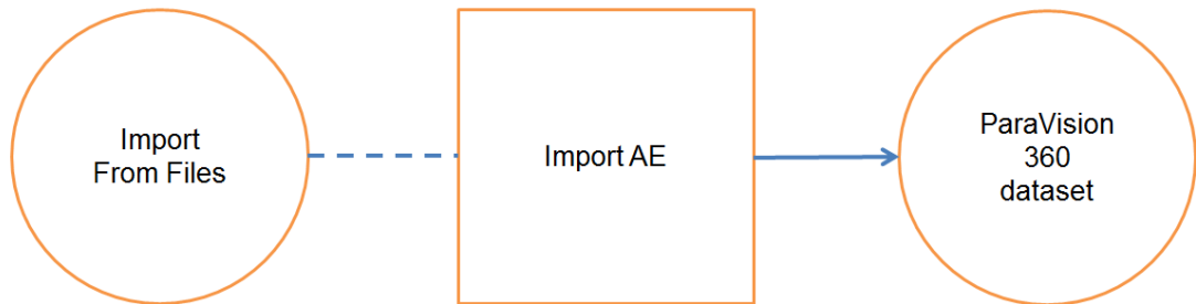
Figure 4.3: Implementation Data Flow Diagram for DICOM Import
